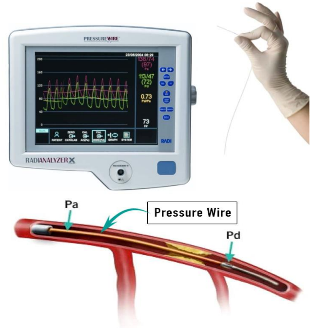
Figure 1: Schematic diagram of FFR Wire and measuring coronary artery pressures distal (Pd) and proximal (Pa) to the stenosis (3)
